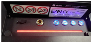
Fig. 9-55 LED strip after detecting unmet safety conditions
