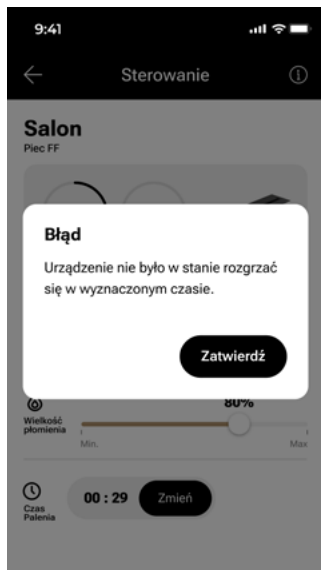
Fig. 9-46 Message about a possible failure of the heating block heaters
