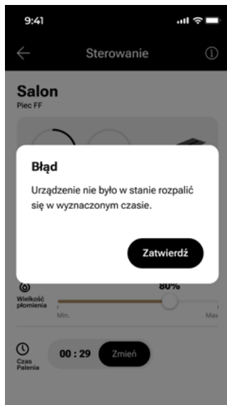
Fig. 9-47 Message about a possible failure of the ignition rod
