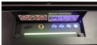
Fig. 9-52 LED strip during the device ignition
