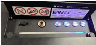
Fig. 9-54 Indication of approximately 5% fuel in the tank
